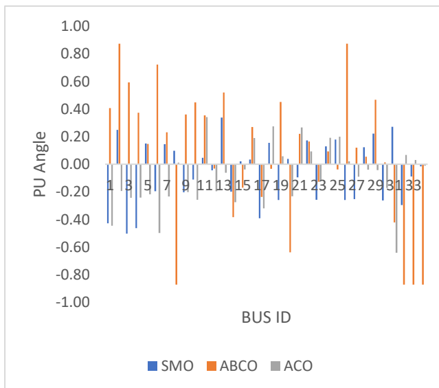
Fig. 4: Busbar Voltage-Angular Magnitude in PU
