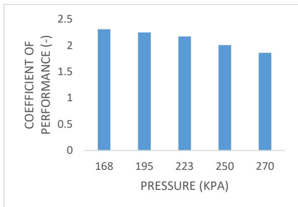
**Figure 12: Effect of Pressure on Coefficient of Performance of the Propane Pre-Cooling Unit**
