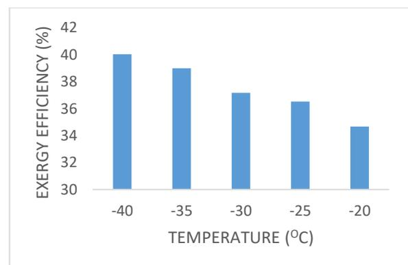
Figure 11: Exergy efficiency for the propane pre-cooling cycle
