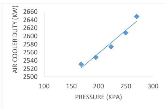
Figure 9: Effect of Pressure on the Air Cooler Duty
