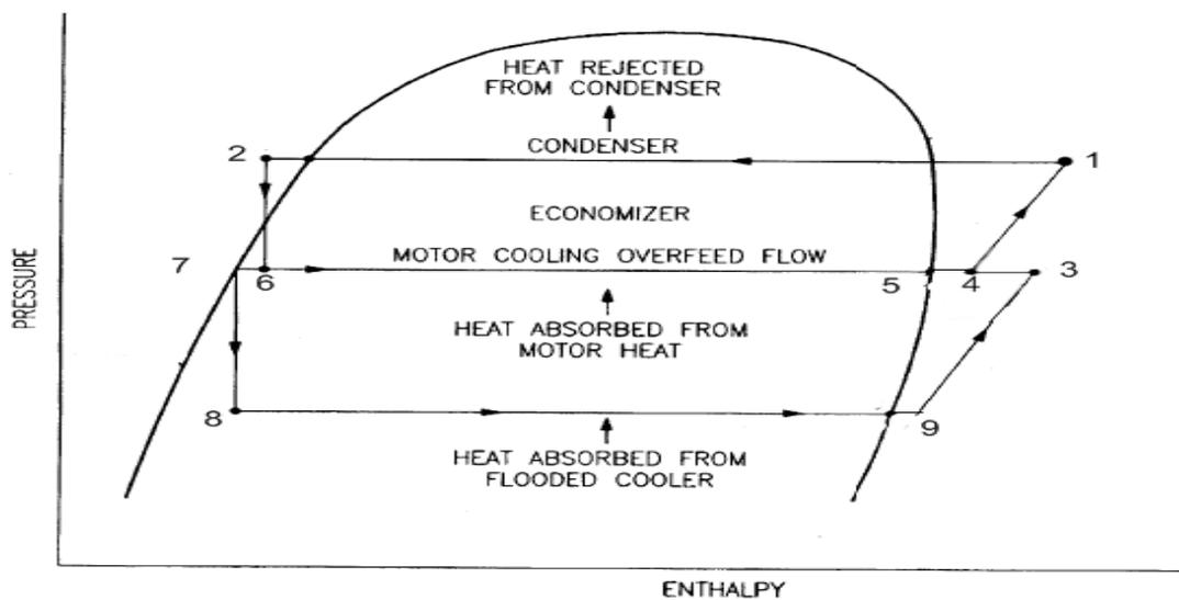
**Figure 2: The Pressure-Enthalpy Diagram of Propane Refrigeration cycle**
