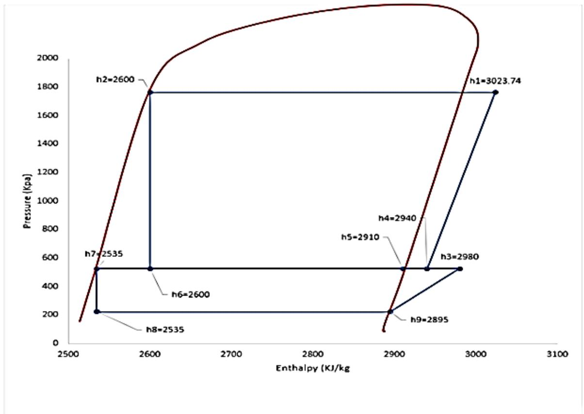
Figure 7: Pressure-Enthalpy (P-h) Diagram for the Propane Refrigeration Loop
