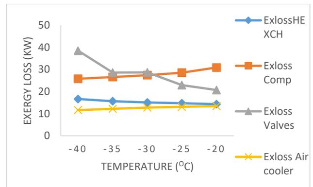
Figure 10: Exergy Loss for each Unit Operation in the Propane Pre-Cooling Cycle
