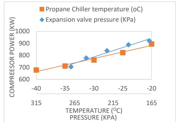
Figure 8: Effect of Pressure on the Compressor Power
