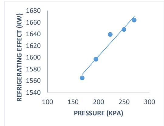
**Figure 13: Effect of Pressure on Refrigerating Effect**
