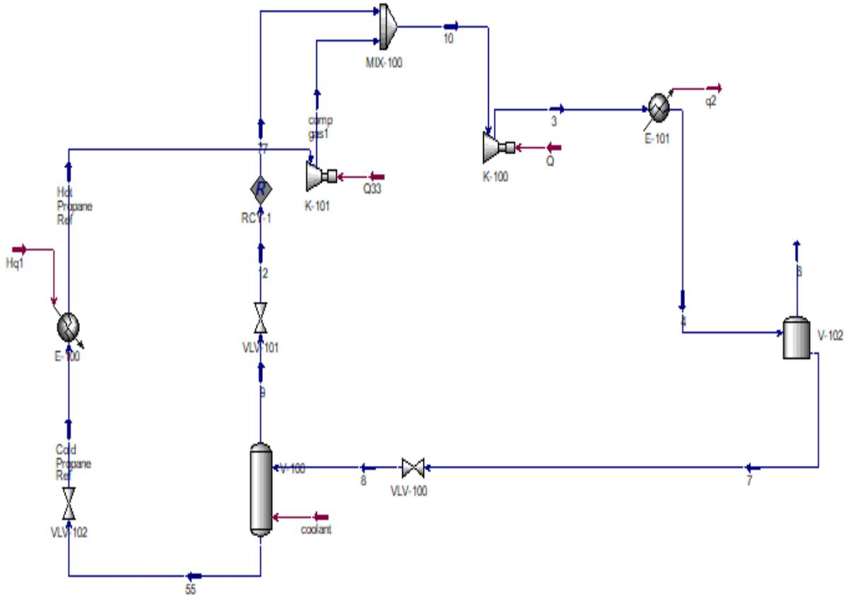
**Figure 1: Propane Refrigeration Unit**
