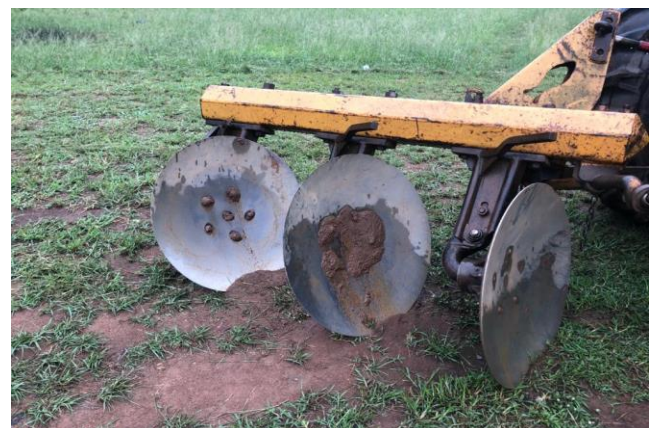
Plate 2: The Disc Plough (Baldan Implementos Agricolas, Brazil) used in this Study
