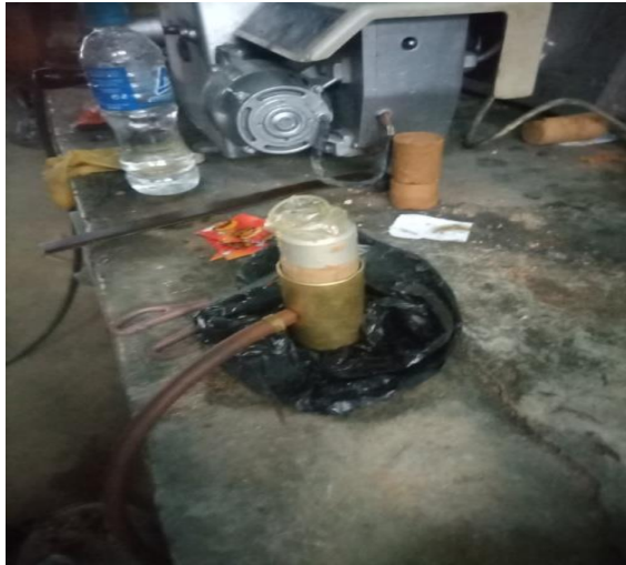
Plate 1: Preparation of the Modified Soil Sample for UCS Test
