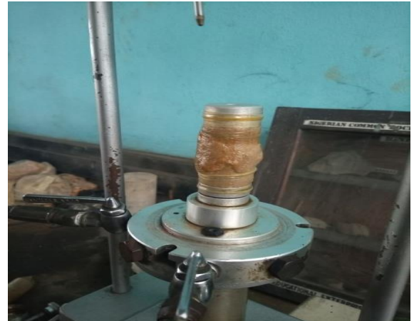
Plate 3: Sample Depicting a Point of UCS Test Failure
