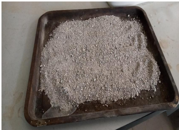
Figure 1. Activated Periwinkle Shell Char
