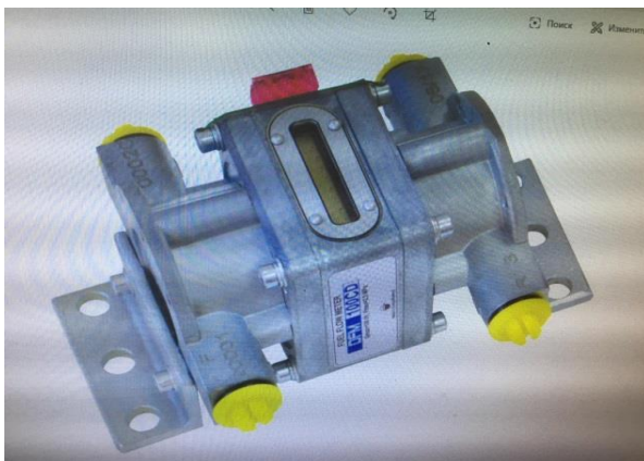
Plate 3: DFM 100CD Fuel Flow Meter (Technoton Engineering, Belarus) used in this Study
