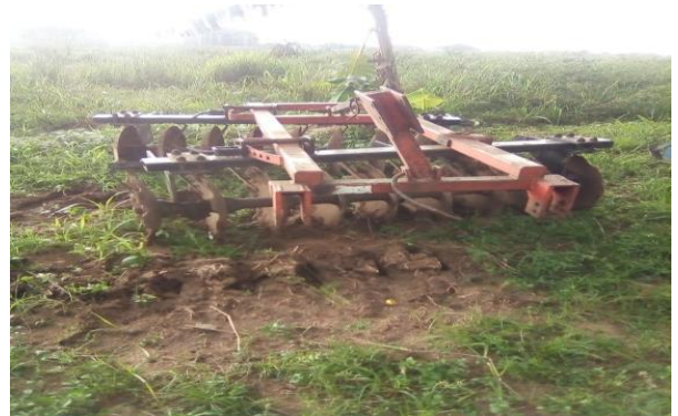
Plate 2: The Disc Harrow (Baldan Implementos Agrícolas, Brazil) used in this Study
