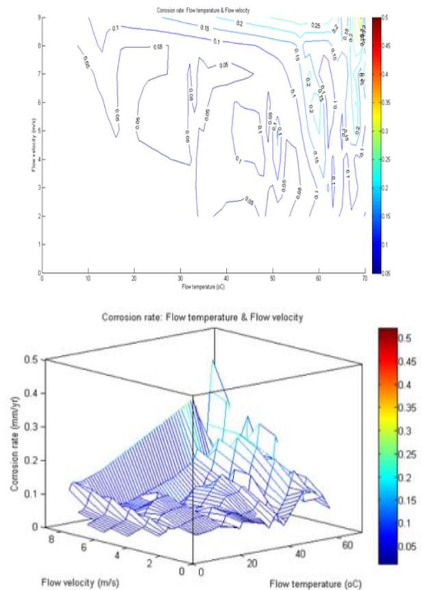
Fig.4: Contour and surface plot of fluid temperature and flow velocity on corrosion rate
