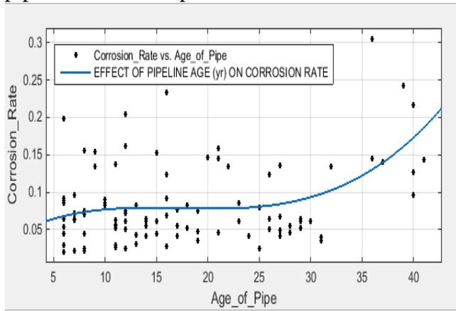
**Fig.5: Effect of pipeline age on corrosion**
