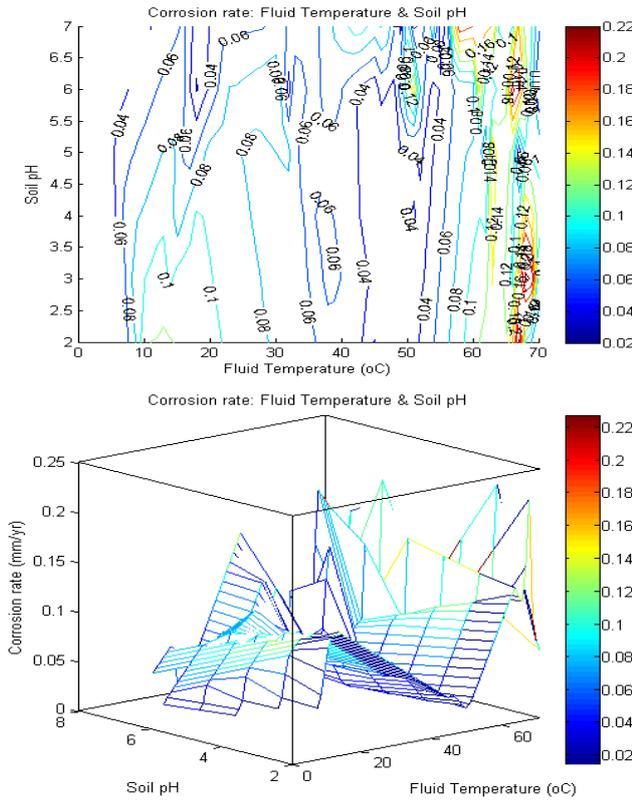
**Fig.8: Contour and surface plots of fluid temperature and environmental pH on corrosion rate**
