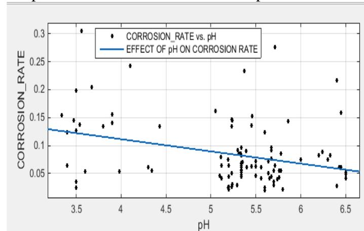
**Fig.7: Effect of environmental pH on corrosion**
