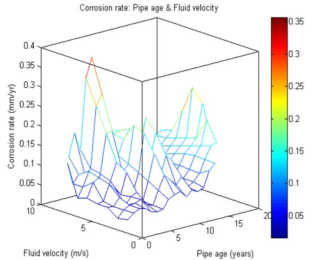
**Fig. 6: Contour and surface plots of fluid velocity and pipe age on corrosion rate**
