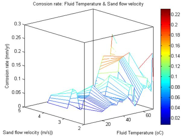
**Fig.12: Contour and surface plots of sand flow and fluid temperature on corrosion rate**
