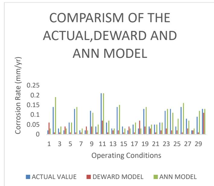
**Fig.13: A comparison of the Actual value, developed ANN model with DeWaard at different operating condition**
