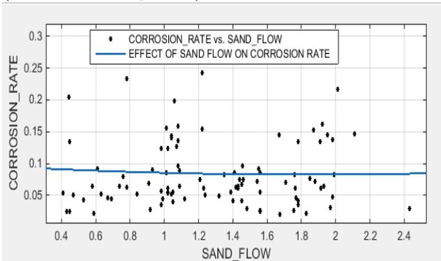
**Fig.11: Effect of sand flow on corrosion**
