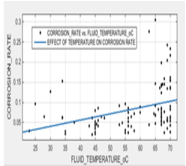
Fig. 3: Effect of temperature on corrosion
