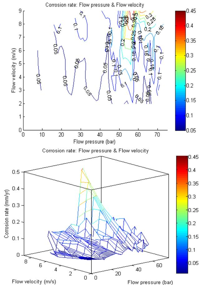
**Fig.10: Contour and surface plot of flow pressure and flow velocity on corrosion rate**
