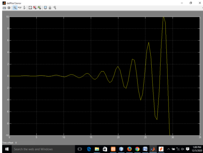
Figure 4: Tie Line Power Deviation (in p.u) with Respect to Time (in seconds) due to Change in Load of Area 1 without any PID Controller.
