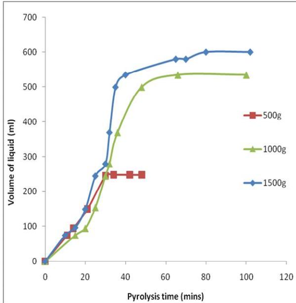
**Fig 5 Variation of volume of liquid produced with respect to pyrolysis time and the quantity of palm kernel shells (Dura)**
