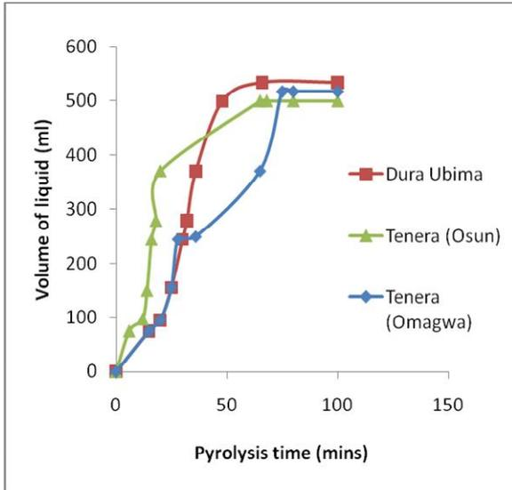
**Fig 3: Volume of liquid produced during pyrolysis by different palm kernel shells with respect to time.**
