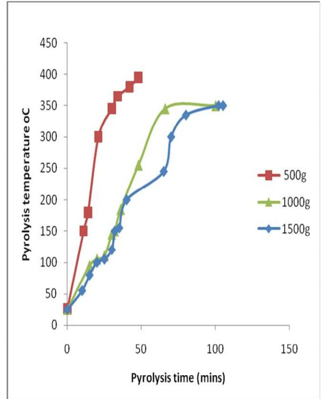
**Fig 4: Variation of product temperature and pyrolysis time on the quantity of palm kernel shell (Dura)**
