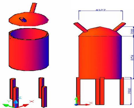
**Fig 6: 3D and first angle autographic view of the batch reactor for PKS.**
