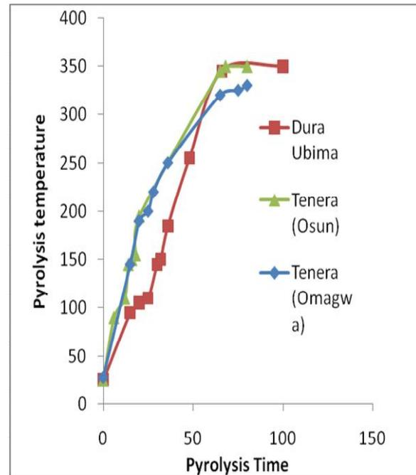
**Fig 2: Product temperature during pyrolysis of palm kernel shells collected from different location with pyrolysis time using different palm kernel shells.**
