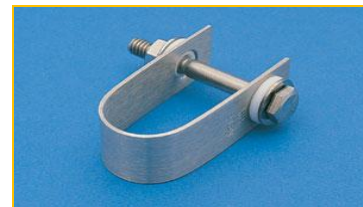
Fig 5: A view of U-bent specimen to a stress level (ASTM G-30, 2016; Metal Sample, 2020)
