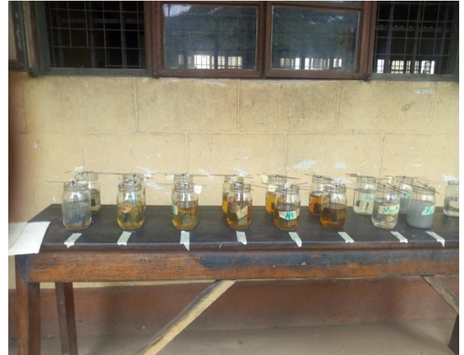
Figure 1 Coupons exposed to corrosion and inhibition at different concentrations
