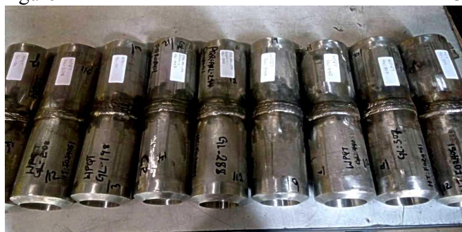
Figure 3: Image of Welded Samples used in the Experiment
