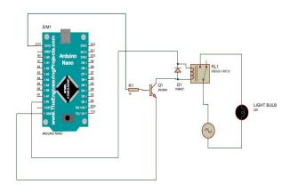
Fig 2: Relay switching Circuit.
