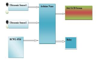
Fig 1: System Component Interaction.
